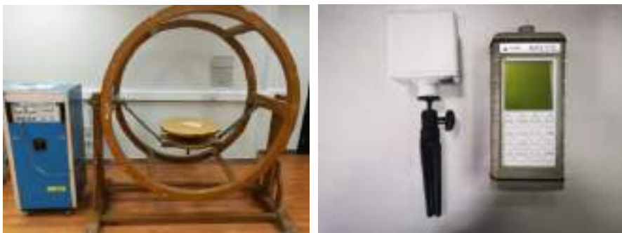
Figure 7. Power-frequency Magnetic Field Experimental Equipment(left) and Teslometer and Standard Probe(right).
