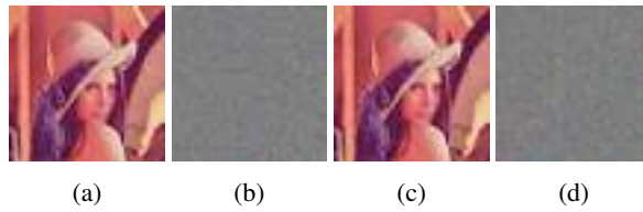
Figure 6. A key sensitivity test is performed on the following images: (a) The original image; (b) The encrypted image; (c) Decrypting the image correctly; (d) Decrypting the image after the key has been changed.
