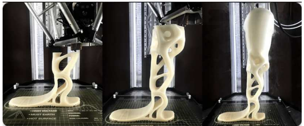
Figure 8. UniLeg Spotlight: the world's first complete 3D-printed below-knee prosthesis solution [8].
